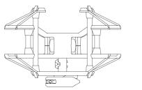
Shock mount that reduces low-frequency rumble and structure-borne noise
