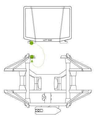
Mount the shock mount onto a stable microphone stand. Open the fixture of the shock mount. Put the tube microphone in the shock mount. The tube window indicates the default front. Lock the fixture.
